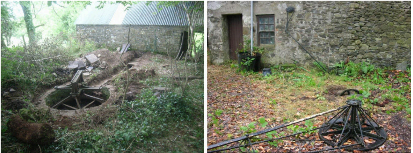
Figure 7: Images of two open-air horse gins in Northern Ireland that show some of the mechanism. Left: Excavation of the open-air horse gin at Creevyloughgare, Saintfield, County Down, showing the subsurface structure including the underground trough that carried the drive shaft to the adjacent barn. 12 Right: The arm of the open-air horse gin at Greenhill, Annahilt, County Down, also with parts of the mechanism visible half-way back towards the building and at the base of the building itself. This horse gin drove a creamery churn and the linear diagonal and vertical structures at centre on the farm building wall are parts of the mechanism to transfer power to an overhead drive at the churn. 13
