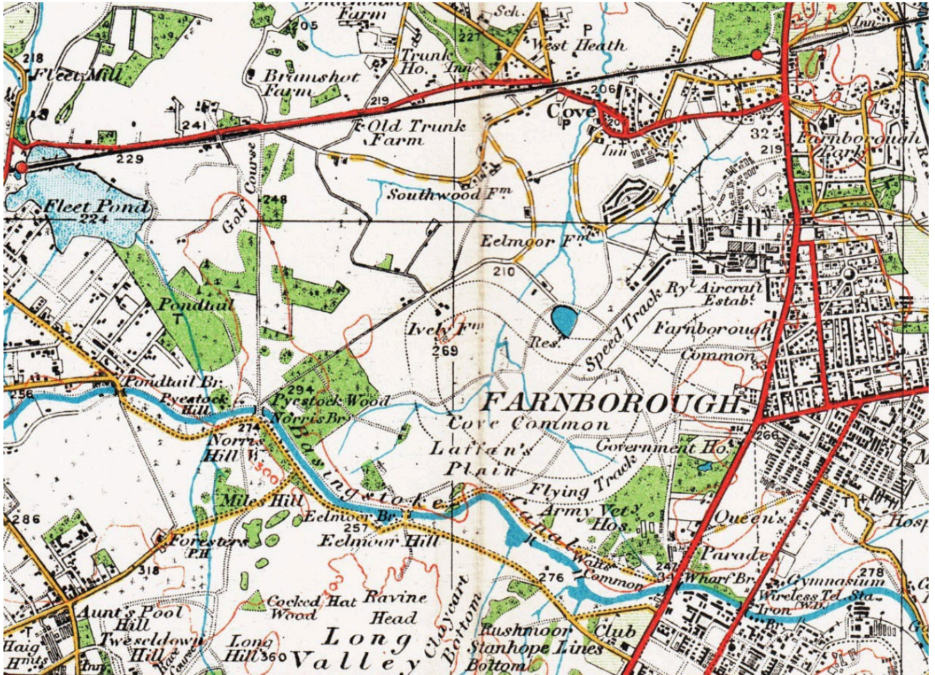
Figure 10: Popular Sheet 114 'Windsor' of 1920 showing RAE, its railway, and flying tracks in detail.
