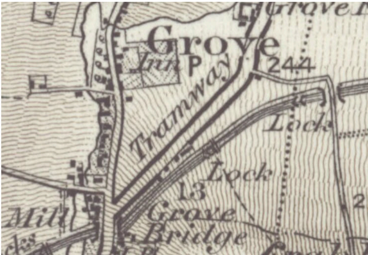
Figure 10c: OS Revised New Series one-inch 'Hills' edition 1903 showing the absence of a tramway symbol on the road to the station, but with the 'Tramway' text beside the road.
