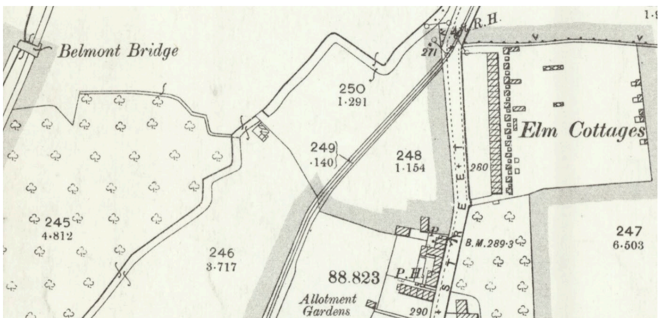
Figure 8a: OS 25-inch 1878 showing the deviation of the Wantage Tramway from the roadside to its own reservation near Elm Cottages
