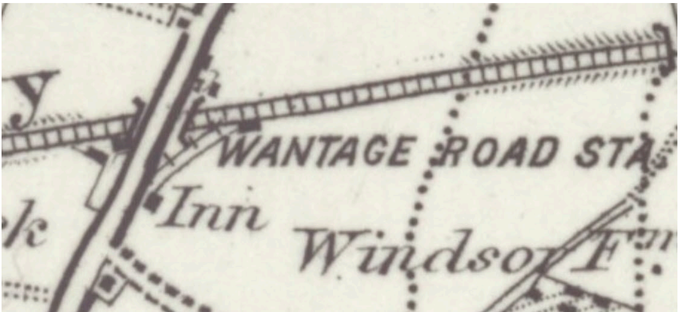
Figure 10a: OS one-inch Revised New Series 'Outline' edition 1895 showing the tramway symbol for the off-road approach to Wantage Road Station (GWR).
